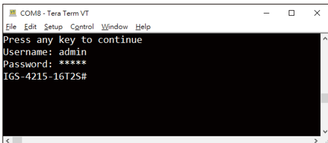
Figure 4-2: Industrial Managed Switch Console Login Screen
